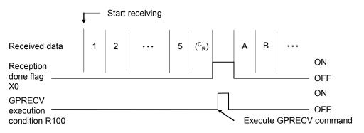
• When the GPRECV command is executed, data are copied into the specified area, and the reception done flag (X0, X1, X2) turns OFF. The reception done flag (X0, X1, X2) turns OFF when the I/O refresh is executed at the beginning of the subsequent scans.
