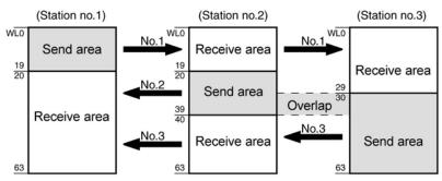
• The allocations shown below are not possible, neither for link relays nor for link registers.
