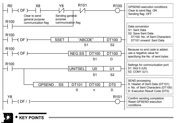
When you do not wish to add the terminator (end code), use a negative value for specifying the No. of sent data in GPSEND command. Select "SS" for operation unit.
