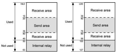
• If all the link relays are used in the PLC link 0 area, set the link relay range of use to "64" (64 words), and all the link register range of use to "128" (128 words).
