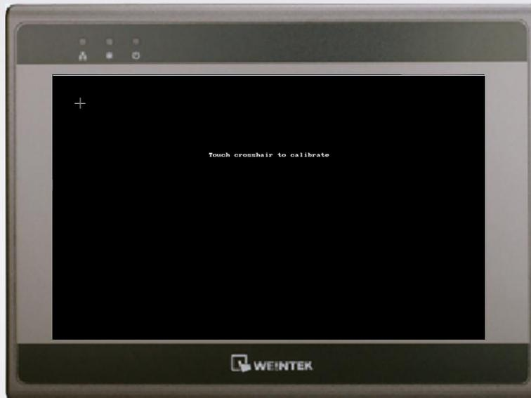
**Step 3.** After all the calibration points have been touched, a pop-up window is displayed and begins countdown from 10 seconds. During the 10-second countdown, the user can touch the screen to check the calibration result. If the result is incorrect, touch the [RETRY] button to restart. If the result is correct, touch the [OK] button within 10 seconds, the calibration data will be saved to the system; otherwise, the calibration will restart.
