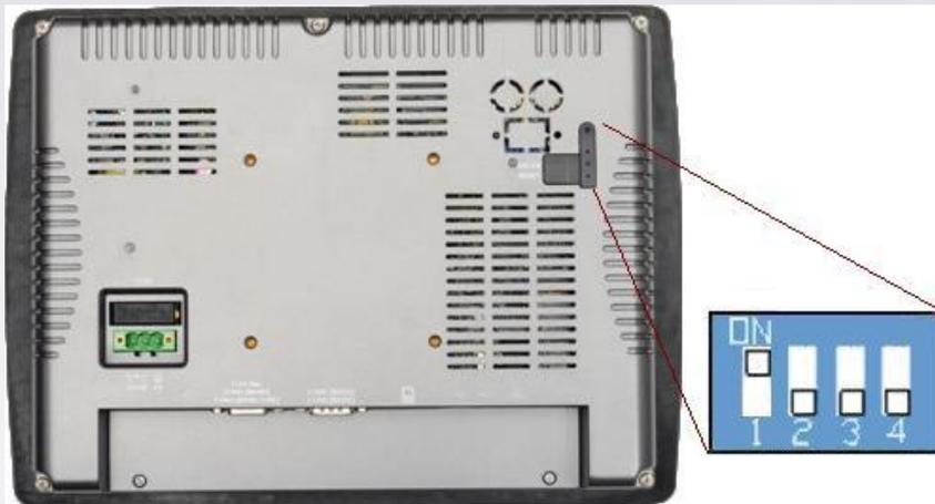
**Step 2.** A “+” sign appears on the screen, touch the center of the sign, after all 5 signs are touched, “+” disappears and the touch screen parameters will be stored in HMI system.
