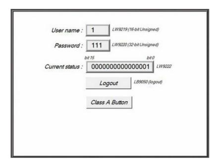
The user 1 is permitted to use object with class A. Consequently, [SB\_0] appears and allows user to operate. Now, bit 0 in [LW9222] becomes 1.
