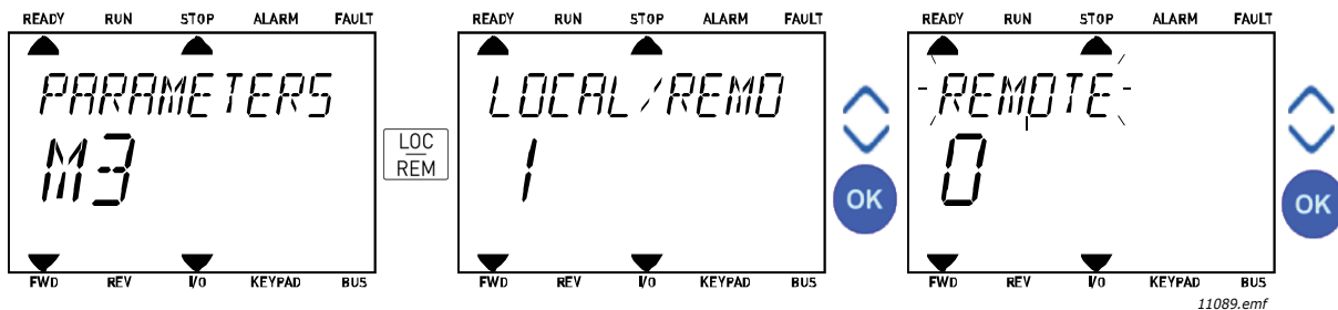
Figure 10. Changing control places
