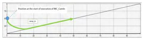
The final StartMode is determined by MC\_CamIn.StartMode and MC\_CamTableSelect.SlaveAbsolute.
