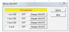
2. Set the servo to on/off by clicking the [Change ON/OFF] for the equivalent axes. If the servo is on for the 1 axis to 3 axis, the setting is as below.
