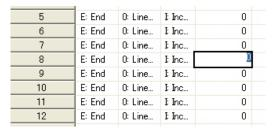
However, in the column with the combo box as below, the data item can be set only by inputting the initial character on the keyboard. For example, input [C] directly in the column of the pattern. Then the data item will be [C: Continuance point]. Also, it is possible to select with the arrow keys after the input is enable.
