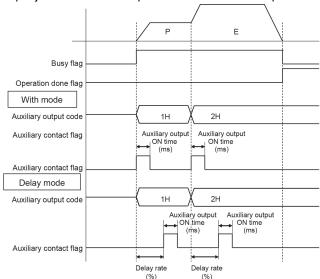
**Note:** The auxiliary output code is stored when the positioning starts regardless of the type of auxiliary output modes (With mode or Delay mode).
