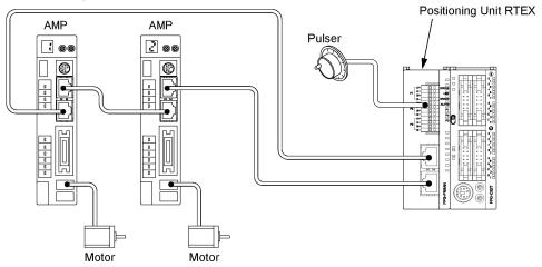
The FP $\Sigma$  positioning unit RTEX is installed in the slot 0. Also, the axes 1 and 2 are designated as the axes used, and the linear interpolation of 2 axes is designated as a sample operation, by the Configurator PM in advance.
