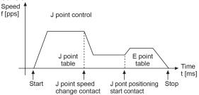
Also, the speed can be changed during the J point control. For changing the speed, turn the J point speed change contact ON after changing the following parameters in the parameter setting area.
