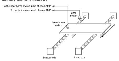
DOG method: Connect the near home switch input of the master axis to the salve axis, too. Limit method: Connect the limit switch input of the master axis to the salve axis, too.
