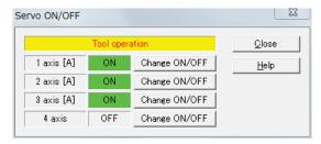
3. Click [Close] to close this dialog after completing the servo ON for the axes operated in the tool operation. The tool operation dialog is automatically shown once the dialog is closed.
