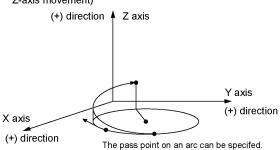
The interpolation speed is the tangential velocity of arc.
