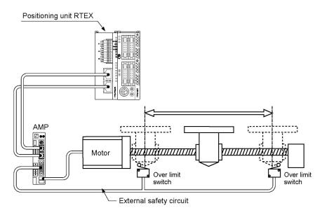
Install over limit switches as shown above.
