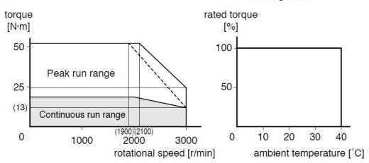
Dotted line represents the torque at 10 % less supply voltage.
