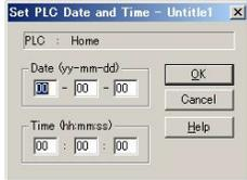
The above steps display the "Set PLC Date and Time dialog box" shown at the left. Input the date and time, and click on the "OK" button.
