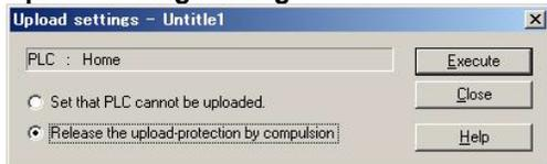
Select “Release the upload-protection by compulsion”.
