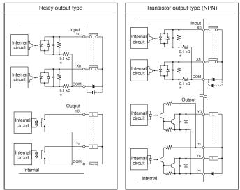
Note: For transistor output types, make sure that the externally supplied voltage between the (+) and (-) termina is between 21.6 and 26.4 V DC. \* for expansion unit: 5.1 k  $\Omega$
