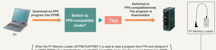
to FP0R, FP0R will automatically be set into FP0-compatible mode. For the program transport to FP0R, use FP Memory Loader Ver. 2.0 or later. (Ver. 1.1 and earlier versions are not compatible with FP0R.)
