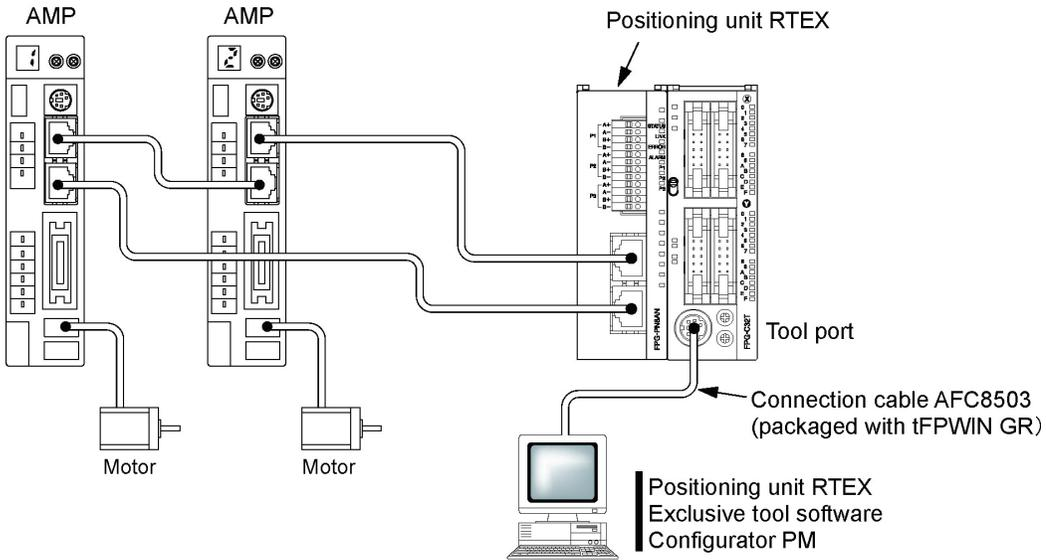
Install the Configurator PM on a computer, and connect it to the tool port of the FP $\Sigma$  control unit like the above example as well as a programming tool.
