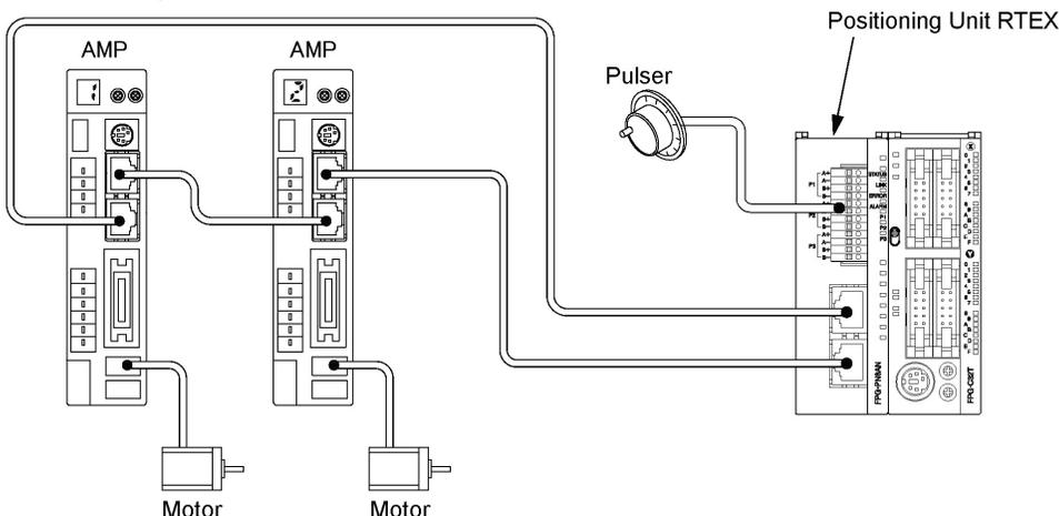
The FPΣ positioning unit RTEX is installed in the slot 0. Also, the axes 1 and 2 are designated as the axes used, and the linear interpolation of 2 axes is designated as a sample operation, by the Configurator PM in advance.
