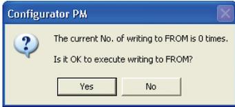
Clicking [Yes] indicates the following dialog and save the setting data in the FROM (Flash Memory) in the unit. The saved setting data is automatically read when the power supply of the PLC turns on.
