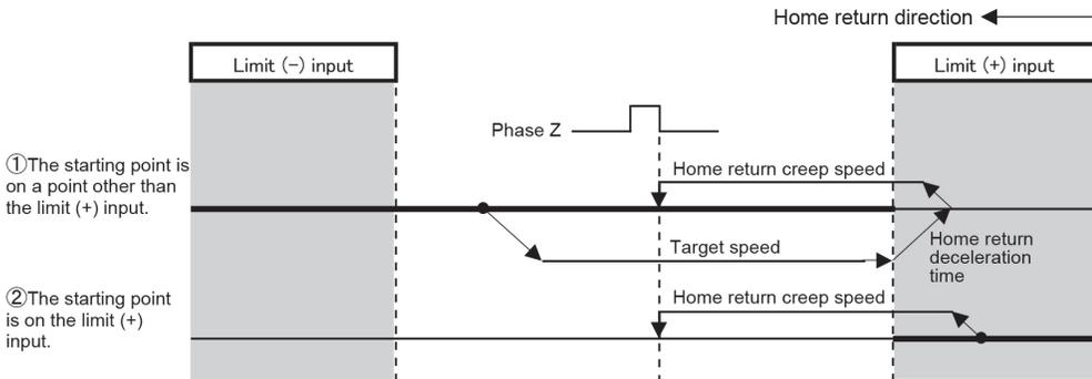
**Limit method 2 (Edge detection of limit switch)**
