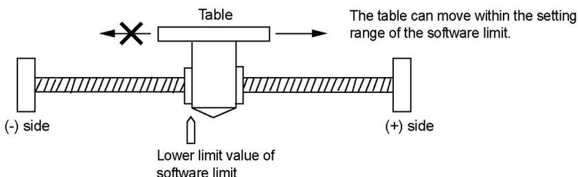
Whether the software limit is set to be available or not can be specified individually for the positioning control, JOG operation and home return each. For example, it is possible to set the limit software to be invalid only in the home return operation.
