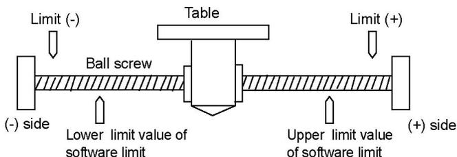
When exceeding the setting range of the software limit (upper and lower limit values), an error occurs, and the deceleration stop is executed. It is necessary to clear the error and move the motor into the range of the software limit using an operation such as JOG operation after the stop.
