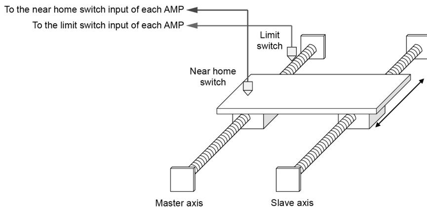
DOG method: Connect the near home switch input of the master axis to the slave axis, too.
