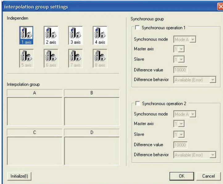
6. To perform the synchronous operation, check the synchronous operation and specify each setting.
