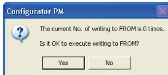
Clicking [Yes] indicates the following dialog and save the setting data in the FROM (Flash Memory) within the positioning unit RTEK. The saved setting data is automatically read when the power supply of the PLC turns on.
