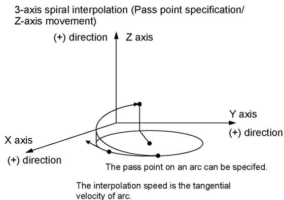
When the X axis and Y axis is the moving axes, each axis in the above diagram is replaced.
