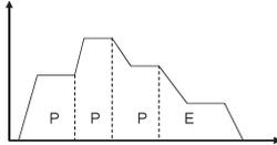
When setting the dwell time to 0 for the E point control that is the last of the positioning control, the positioning unit processes the E point control as the P point control, and completes the operation after repeating the positioning control for 3 times without stopping the operation.
