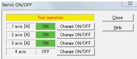
3. Click [Close] to close this dialog after completing the servo ON for the axes operated in the tool operation. The tool operation dialog is automatically shown once the dialog is closed.
