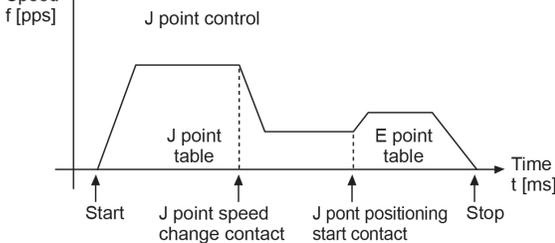
Also, the speed can be changed during the J point control. For changing the speed, turn the J point speed change contact ON after changing the following parameters in the parameter setting area.
