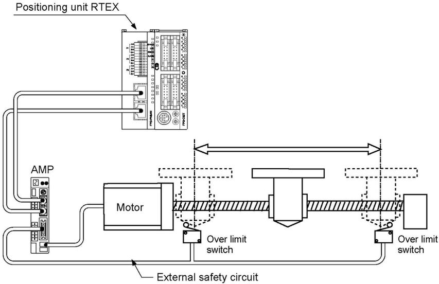
Install over limit switches as shown above.
