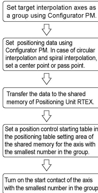
The procedures to set the positioning data and to start the position control are the same for the E point control, P point control and C point control. The operation of each control is determined according to the contents of the positioning data to be set.
