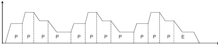
When setting the dwell time to a number other than 0 for the E point control that is the last of the positioning control, the positioning unit processes the E point control as the C point control, and execute the positioning control again after stopping the operation for the dwell time (ms). The positioning unit completes after repeating the positioning control for 3 times.
