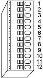
Input terminals of pulser input connector
