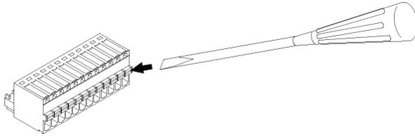
(3) Insert the wire into the connector until it stops with pressing the orange switch.
