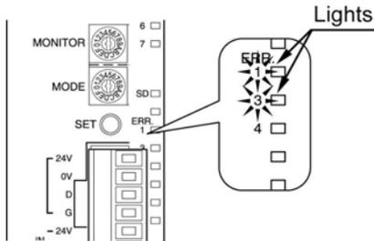
**(1) The line between D and G is short-circuited. Eliminate the cause of the error.**
