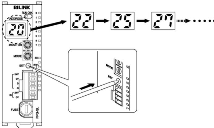
To check error addresses other than the one that is displayed, set the “RUN/CHK.” selector switch to the “CHK.” position, and press the system SET button.
