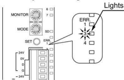
There is no terminal resistance, or noise is added on the wiring. Connect the wiring correctly, and eliminate the noise.
