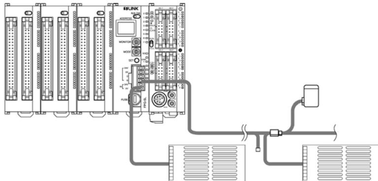
③ Main unit power supply ← ..... ② S-LINK main power supply ← ..... ① Local power supply
