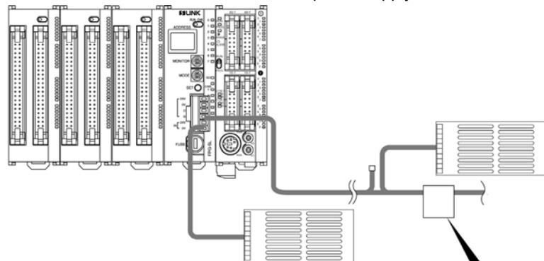
③ Main unit power supply ← ..... ② S-LINK main power supply ← ..... ① Booster local power supply
