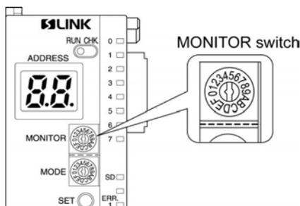
As shown in the table below, eight addresses are assigned to each numeric value on the MONITOR switch, in sequential order. Select the numeric value that includes the address to be confirmed.
