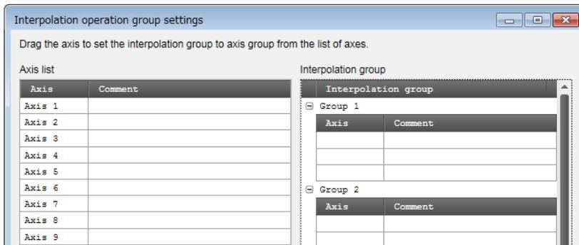
5. Drag the line to be allocated for interpolation to the interpolation group field.
