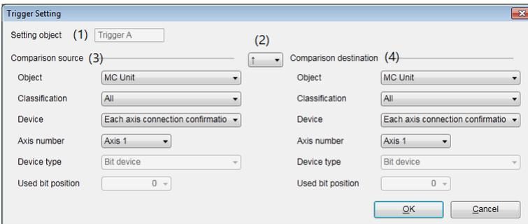
4. Select trigger setting conditions, and press the [OK] button. The detailed information of trigger conditions is displayed.
