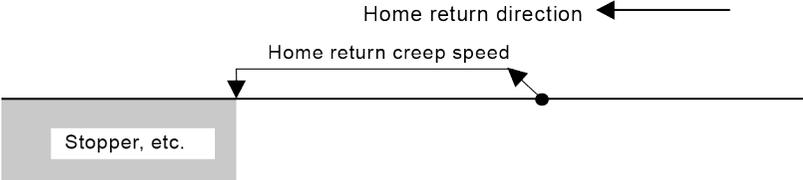
■ **Stop-on-contact method 2 (Stop-on-contact + Z phase)**
