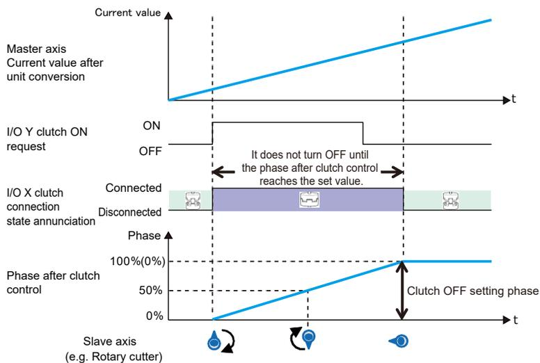
(Note 1) The above figure shows the case where both the clutch ON request and clutch OFF request are set to "Level". Also, either "Rise" or "Fall" can be selected.
