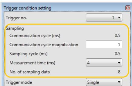
2. Select a trigger number, sampling condition, trigger mode, trigger position and trigger condition.
