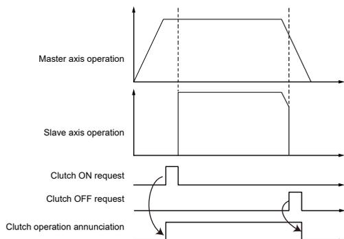
(Note 1) The above figure shows the case when selecting "Direct" for the connection method and "Leading edge" for the clutch ON and OFF requests.
