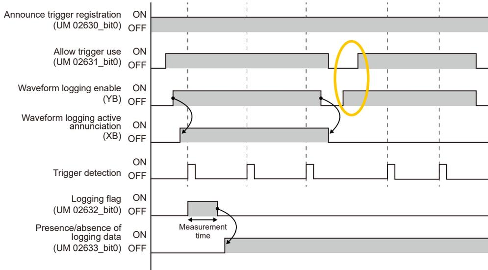
(Note 1) If the waveform logging enable (YB) flag turns on before turning on "Allow Trigger Use (UM02631)", the logging operation will not be executed.
