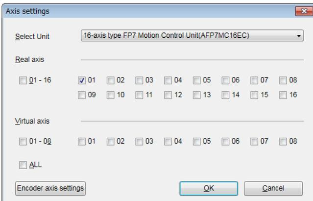
(This is the 16-axis type. For the 32-axis and 64-axis types, see "P.4-8".)
