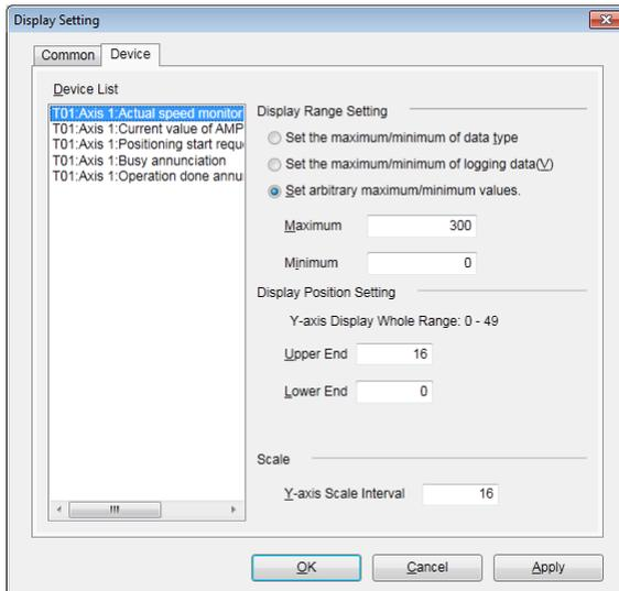
(Note 1) In Scale field, enter an interval between the scales of Y axis by grids. Range: 1 to (Upper end - Lower end)
