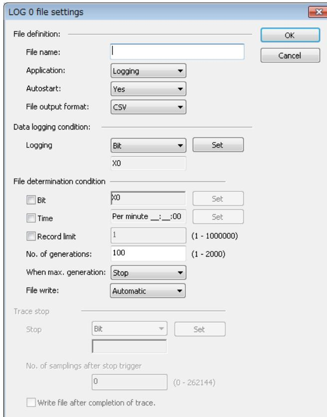
4. Set information in each field of File definition, Data logging condition and File determination condition.
