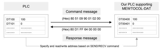
Note: The above figure indicates the data part of MEWTOCOL-DAT. In communication via LAN, a header including size information of the sent data is added.
