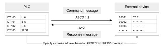
Note: The above figure indicates the data part. In communication via LAN, a header including size information of the sent data is added.
