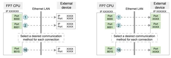
Note) Circled numbers in the figure above indicate examples of allocation of connection numbers.
