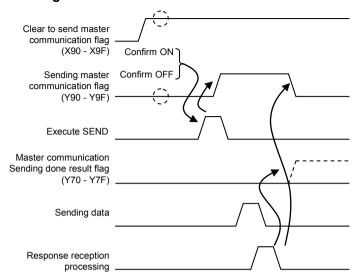
Conditions to enable execution of SEND command Clear to send flag (X90 - X9F): ON Sending flag (Y90 - Y9F): OFF
