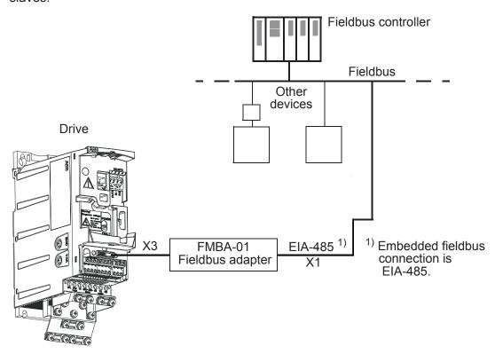
The drive can be set to receive all of its control information through the fieldbus interface, or the control can be distributed between the fieldbus interface and other available sources, for example, digital and analog inputs.
