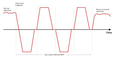
The pump cleaning (anti-jam or anti-ragging) function uses a programmable sequence of forward and reverse rotations of the pump to shake off and remove any build-up of rags on the impeller.
