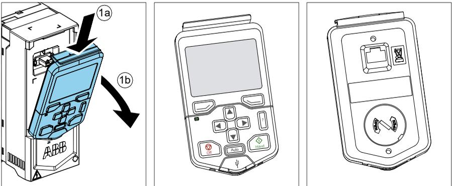
To reinstall the control panel, put the bottom of the container in position (1a), press the retaining clip at the top (1b) and push the control panel in at the top edge (1c).
