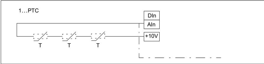
**Note:** It is important to ensure that the DI used for this is not configured to start any action.
