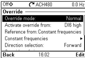
Select Normal or Critical Override mode in **Menu > Primary settings > Override > Override mode**. Normal follows the programmed number of fault resets while in Override mode. Critical allows for infinite number of fault resets. Disabled indicates that Override is not being used.
