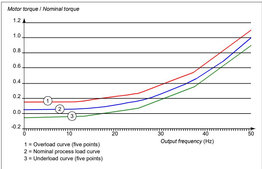
An overload warning and/or fault can be set to occur if the monitored signal stays continuously over the overload curve for a defined time. An underload warning and/or fault can be set to occur if the monitored signal stays continuously under the underload for a defined time.
