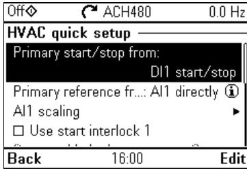
Use the **HVAC quick setup** submenu to go through the most important settings (basic setup and basic operation) at start-up if you do not want to do it with the assistants.
