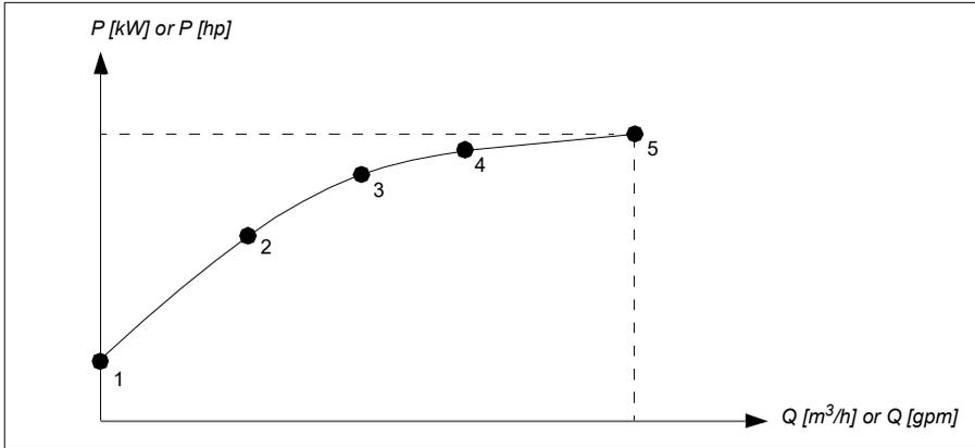
The flow calculated based on HQ or PQ curve is scaled according to the actual speed of the pump. Scaling reference speed is set in parameter [80.21 Flow pump nominal speed](#).
