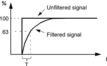
$O = I \times (1 - e^{-t/T})$ <p>I = filter input (step)<br/>O = filter output<br/>t = time<br/>T = filter time constant</p>                                                                                                                                                                                    | 0.0 s      |
