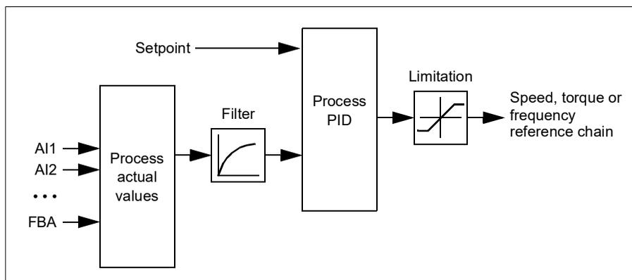
The drive contains two complete sets of process PID controller settings that can be alternated whenever necessary; see parameter [40.57 PID set1/set2 selection](#).
