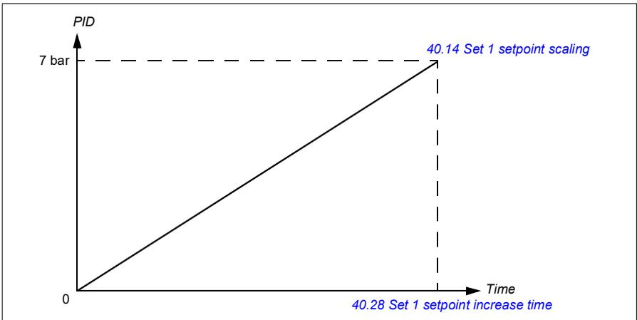
If the pumping system is leaking or is damaged then the setpoint will not reach in time. To detect such a condition, you can enable soft pipe fill supervision to generate a warning or a fault. The time is calculated with the last reference change in parameter [40.03 Process PID setpoint actual](#).
