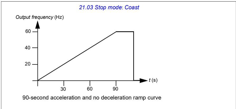
In pump applications, the stop mode is typically set to ramp and the deceleration ramp is used while stopping. Ramping a pump motor to a stop helps prevent issues
