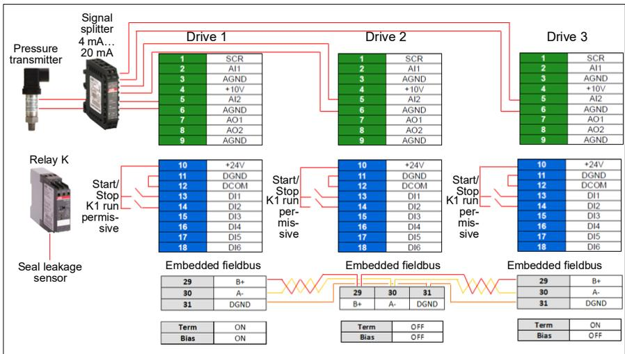
**Note:** If a current signal is used, use a signal splitter to connect the sensor signal to all drives that may take on the master role.
